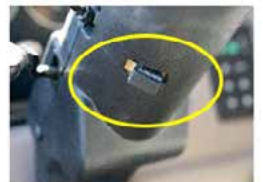
Hazard Warning Flasher
